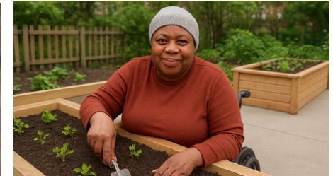
Interactive areas like this garden bed can be raised with a forward approach and knee/toe clearance.
