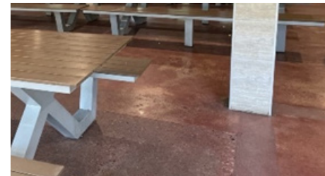
This table provides knee/toe clearance and clear floor space outside the circulation route.
