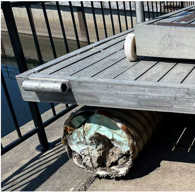
Metal and plastic floats are filled with plastic foam to keep them from sinking when punctured or damaged.
